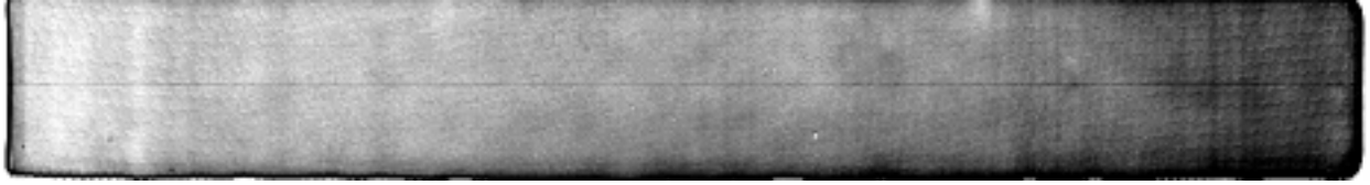
Figure 18. Full field illumination intensity map for FL01 showing the MCP multifibers.
